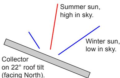
In winter the sun intensity and altitude is lowest, and daylight hours are shortest. The low angle the sun hits the collector surface causes increased reflection, reduced area and input.
