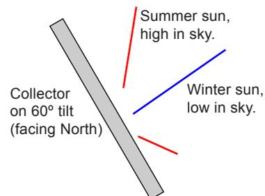
In summer when the sun intensity, altitude and daylight hours is greatest, the input is reduced as the sun angle on the surface reduces its area, with losses by reflection.
